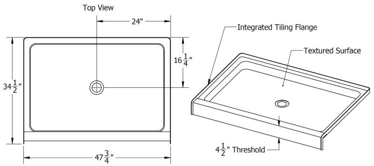
Note: ALL THE MEASUREMENTS ARE IN INCHES & HAVE TOLERANCE OF  $\pm$   $^{1}\!\!/\!\!4''$
