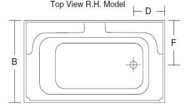
Note: ALL THE MEASUREMENTS ARE IN INCHES & HAVE TOLERANCE OF ± 1/4"
