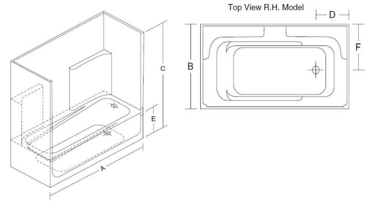
Note: ALL THE MEASUREMENTS ARE IN INCHES & HAVE TOLERANCE OF  $\pm \frac{1}{4}$ "
