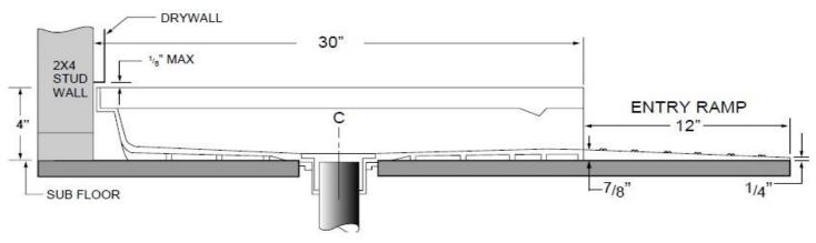
Note: ALL THE MEASUREMENTS ARE IN INCHES & HAVE TOLERANCE OF  $\pm 1/4$ "
