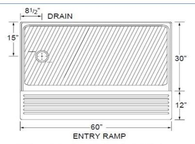
Unit must be placed into a bed of Mortar.
