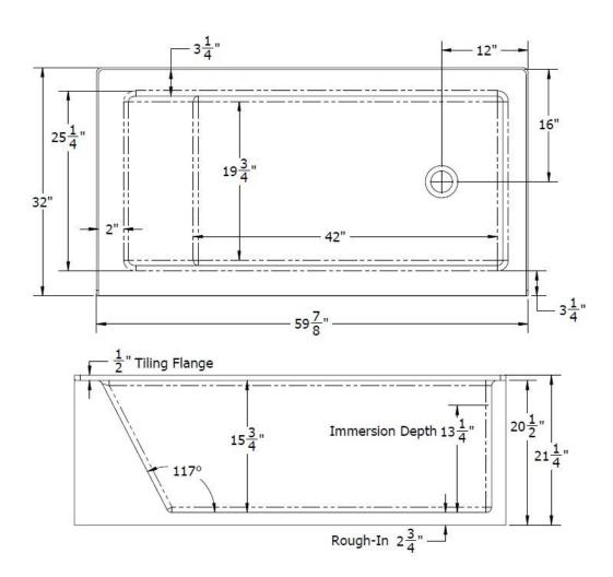
Note: ALL THE MEASUREMENTS ARE IN INCHES & HAVE TOLERANCE OF  $\pm \frac{1}{4}$ "
