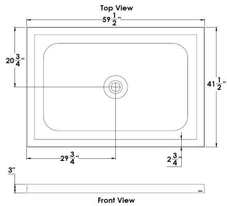
Note: ALL THE MEASUREMENTS ARE IN INCHES & HAVE TOLERANCE OF  $\pm$   $\frac{1}{4}$ "
