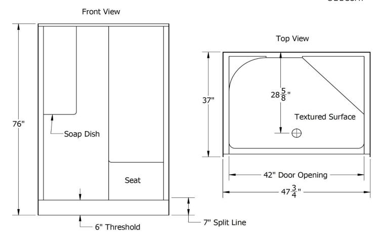
Note: ALL THE MEASUREMENTS ARE IN INCHES & HAVE TOLERANCE OF  $\pm$   $\frac{1}{4}$ "
