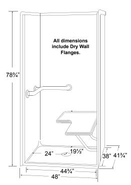
This Shower Stall shall be a VENCO Model No. 4840BFS. Finished surface shall be of a Premium sanitary-grade polyester Gelcoat with a minimal thickness of 15 dry mills and a finished cured Barcol hardness of 80-90. The unit shall have dimensions of  $48" \times 41\%" \times 78\%" 0.D$ .
