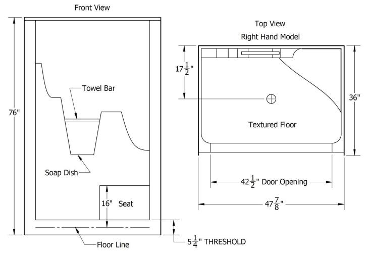
Note: ALL THE MEASUREMENTS ARE IN INCHES & HAVE TOLERANCE OF  $\pm\,1\!4''$
