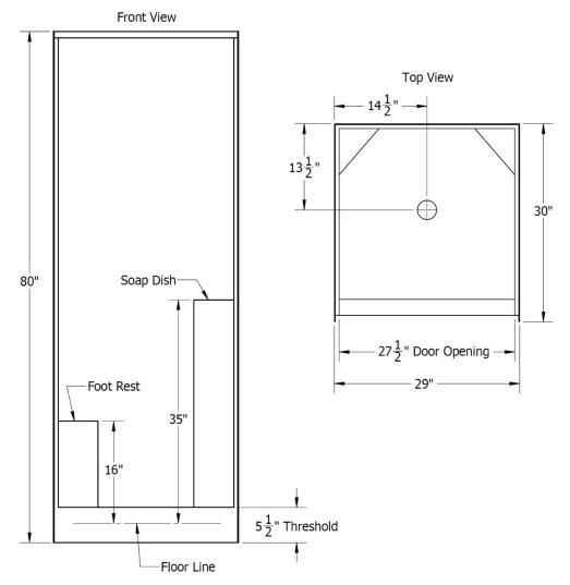
Note: ALL THE MEASUREMENTS ARE IN INCHES & HAVE TOLERANCE OF  $\pm\,1\!/4''$
