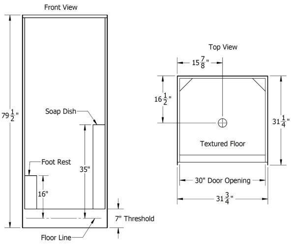
Note: ALL THE MEASUREMENTS ARE IN INCHES & HAVE TOLERANCE OF  $\pm$   $^{1\!/}$
