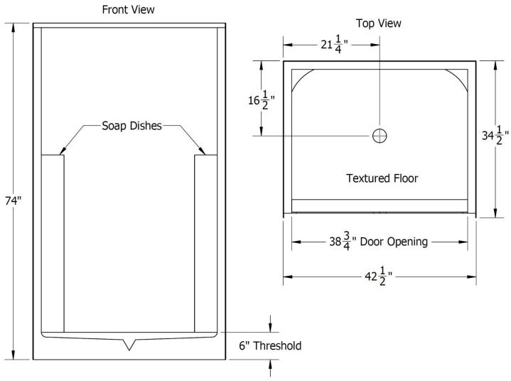
Note: ALL THE MEASUREMENTS ARE IN INCHES & HAVE TOLERANCE OF  $\pm$   $^{1\!/}$
