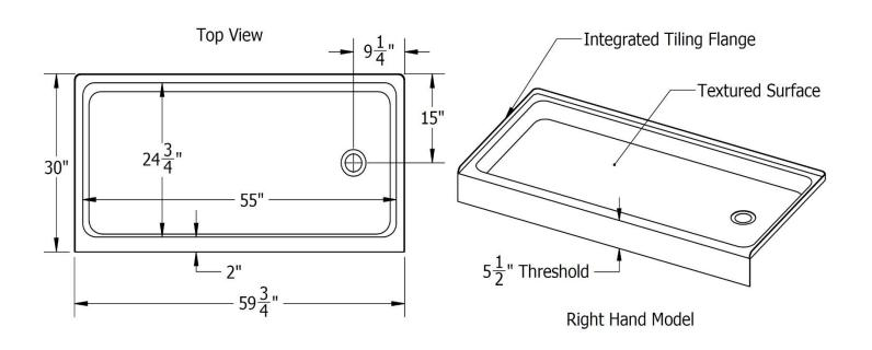
Note: ALL THE MEASUREMENTS ARE IN INCHES & HAVE TOLERANCE OF  $\pm$   $\frac{1}{4}$ "
