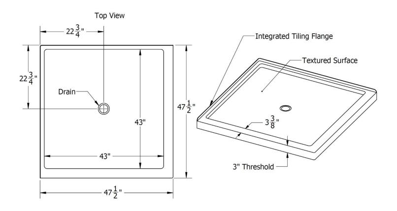
Note: ALL THE MEASUREMENTS ARE IN INCHES & HAVE TOLERANCE OF ± 1/4"
