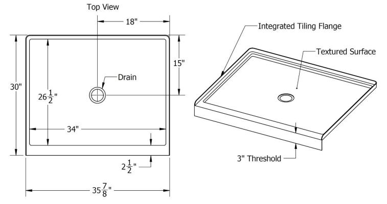
Note: ALL THE MEASUREMENTS ARE IN INCHES & HAVE TOLERANCE OF  $\pm$  <sup>1</sup>/<sub>4</sub>"
