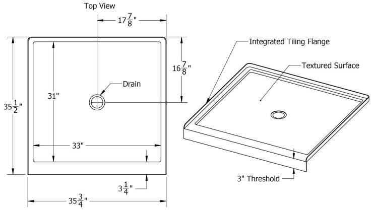
Note: ALL THE MEASUREMENTS ARE IN INCHES & HAVE TOLERANCE OF  $\pm \frac{1}{4}$ "
