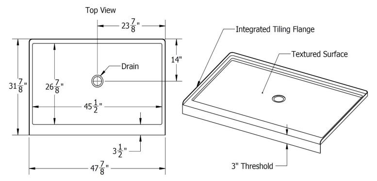
Note: ALL THE MEASUREMENTS ARE IN INCHES & HAVE TOLERANCE OF  $\pm$  <sup>1</sup>/<sub>4</sub>"
