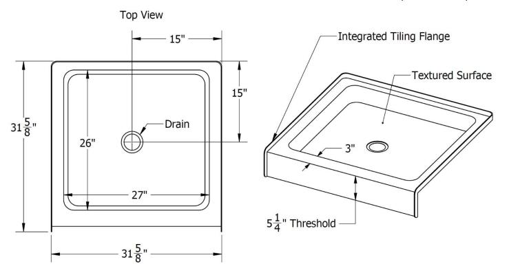
Note: ALL THE MEASUREMENTS ARE IN INCHES & HAVE TOLERANCE OF ± 1/4"
