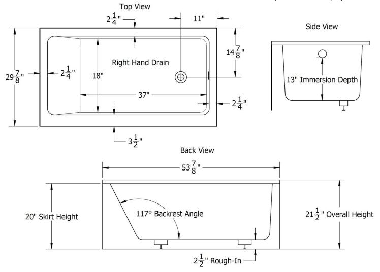
Note: ALL THE MEASUREMENTS ARE IN INCHES & HAVE TOLERANCE OF  $\pm$   $^{1}\!\!\!/4$   $^{\prime\prime}$
