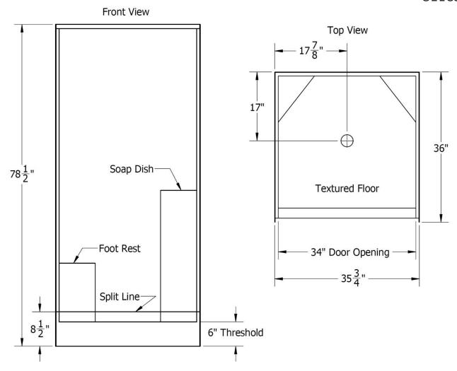
Note: ALL THE MEASUREMENTS ARE IN INCHES & HAVE TOLERANCE OF  $\pm\,1\!/4''$
