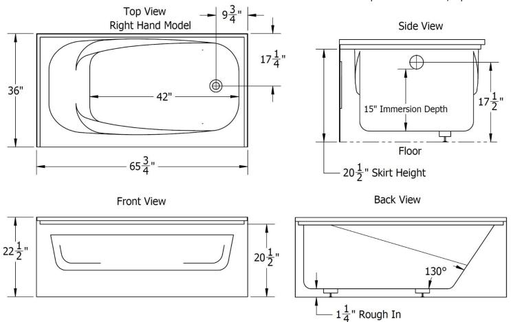
Note: ALL THE MEASUREMENTS ARE IN INCHES & HAVE TOLERANCE OF  $\pm$   $^{1}\!\!\!/^{\prime\prime}$
