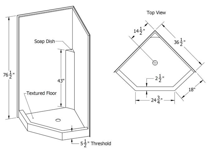
Note: ALL THE MEASUREMENTS ARE IN INCHES & HAVE TOLERANCE OF  $\pm$   $^{1\!/}$
