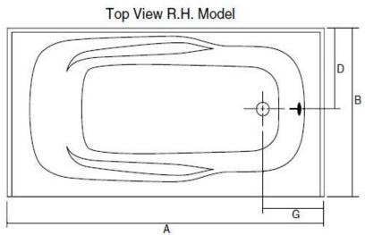
Note: ALL THE MEASUREMENTS ARE IN INCHES & HAVE TOLERANCE OF ± 1/4"
