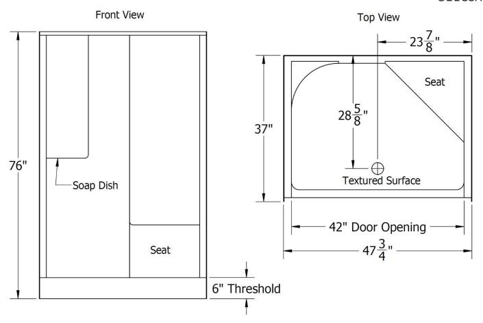
Note: ALL THE MEASUREMENTS ARE IN INCHES & HAVE TOLERANCE OF  $\pm \frac{1}{4}$ "
