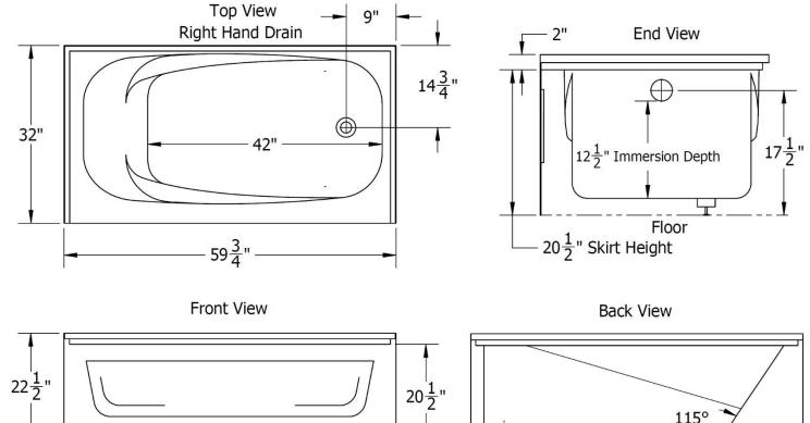
Note: ALL THE MEASUREMENTS ARE IN INCHES & HAVE TOLERANCE OF  $\pm$   $^{1}\!\!\!/^{\prime\prime}$
