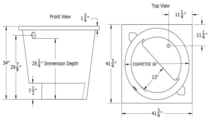
Note: ALL THE MEASUREMENTS ARE IN INCHES & HAVE TOLERANCE OF  $\pm 1/4$ "
