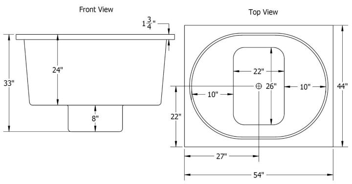
Note: ALL THE MEASUREMENTS ARE IN INCHES & HAVE TOLERANCE OF  $\pm\,1\!/4''$
