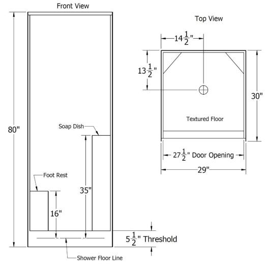
Note: ALL THE MEASUREMENTS ARE IN INCHES & HAVE TOLERANCE OF  $\pm 1/4''$
