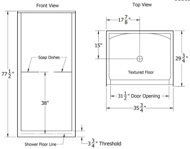
Note: ALL THE MEASUREMENTS ARE IN INCHES & HAVE TOLERANCE OF  $\pm$  1/4"
