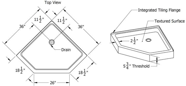
Note: ALL THE MEASUREMENTS ARE IN INCHES & HAVE TOLERANCE OF  $\pm$   $\frac{1}{4}$ "
