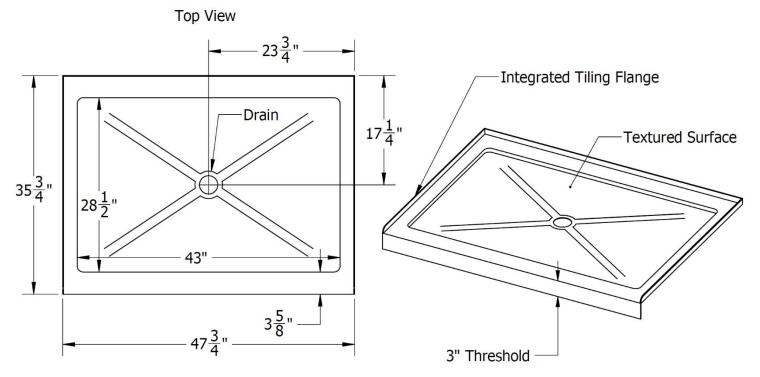
Note: ALL THE MEASUREMENTS ARE IN INCHES & HAVE TOLERANCE OF  $\pm \frac{1}{4}$ "
