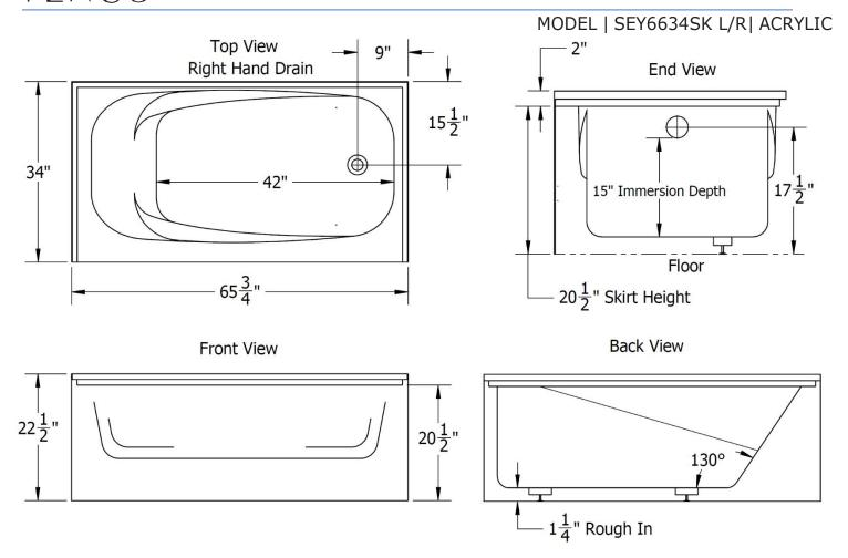
Note: ALL THE MEASUREMENTS ARE IN INCHES & HAVE TOLERANCE OF  $\pm\,1\!/4''$
