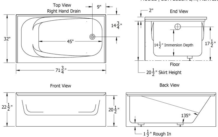
Note: ALL THE MEASUREMENTS ARE IN INCHES & HAVE TOLERANCE OF  $\pm\,1\!/4''$
