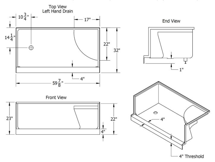
Note: ALL THE MEASUREMENTS ARE IN INCHES & HAVE TOLERANCE OF  $\pm\,^{1}\!\!/\!_{4}{}''$
