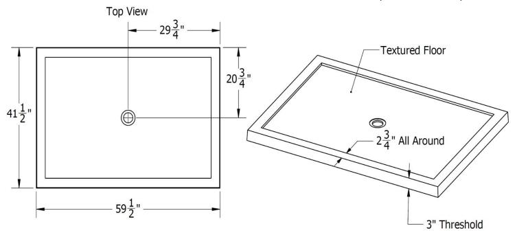
Note: ALL THE MEASUREMENTS ARE IN INCHES & HAVE TOLERANCE OF  $\pm$   $\frac{1}{4}$ "
