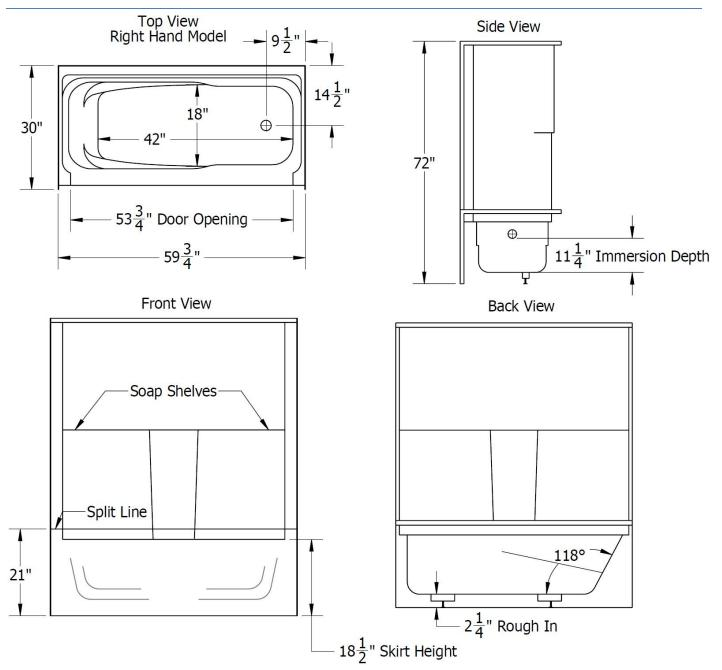
Note: ALL THE MEASUREMENTS ARE IN INCHES & HAVE TOLERANCE OF  $\pm\,1\!/4''$
